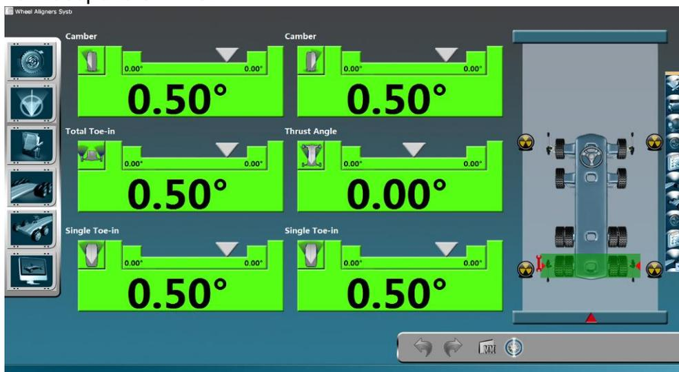
Figure 3-26 Present Rear Axle Adjustment Screen
