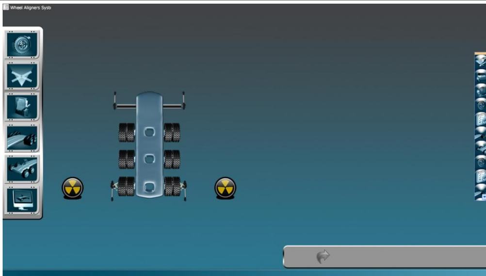
Figure 3-36 Trailer Run out Compensation
