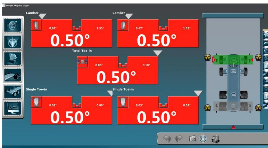
Figure 3-28 Present Front Axle Adjustment Screen
